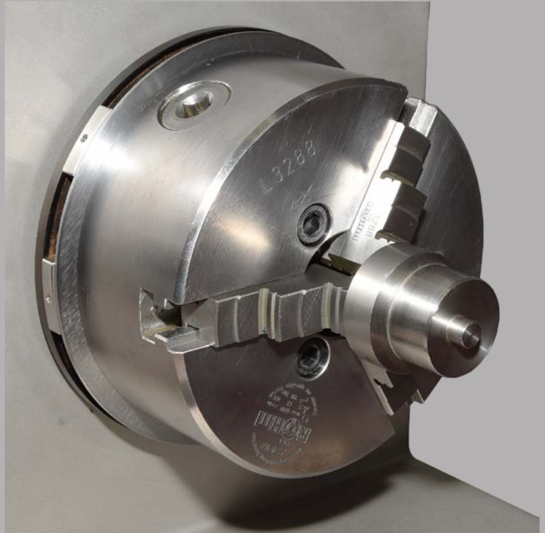
MPM balancing ring with balancing segments: 3.WRS.xxx Patented
