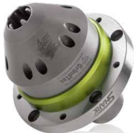
With the SHARK, the clamping jaws are in the same axial position at all times. Due to the uniquely newly developed solid jaw guide, the wobble can be reduced to a minimum. Together with the high concentricity and repeatability, as well as low interfering contours, you achieve process reliability and best results even with difficult processes. During operation, the chuck is cleaned with active sealing air. This prevents contamination and maintains absolute precision over the long term.
